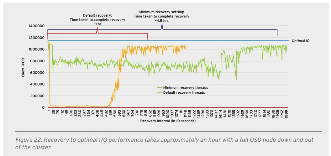
Figure 22. Recovery to optimal I/O performance takes approximately an hour with a full OSD node down and out of the cluster.
