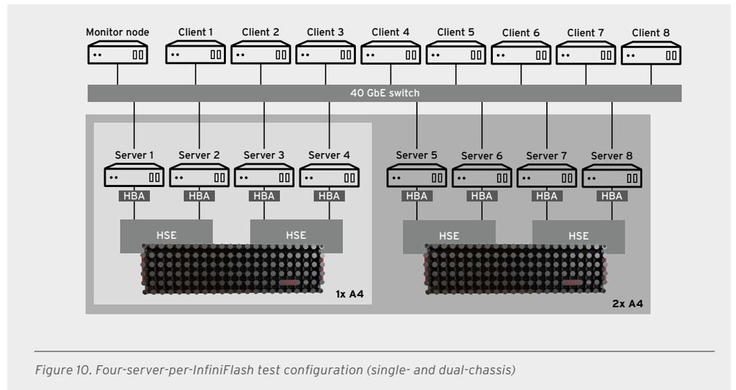
Figure 10. Four-server-per-InfiniFlash test configuration (single- and dual-chassis)
