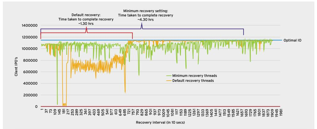
Figure 23. Replacing a full OSD node (13.6TB of data) requires roughly 1.3 hours for the cluster to return to optimal I/O performance.
