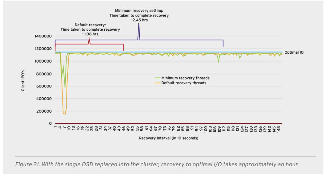
Figure 21. With the single OSD replaced into the cluster, recovery to optimal I/O takes approximately an hour.
