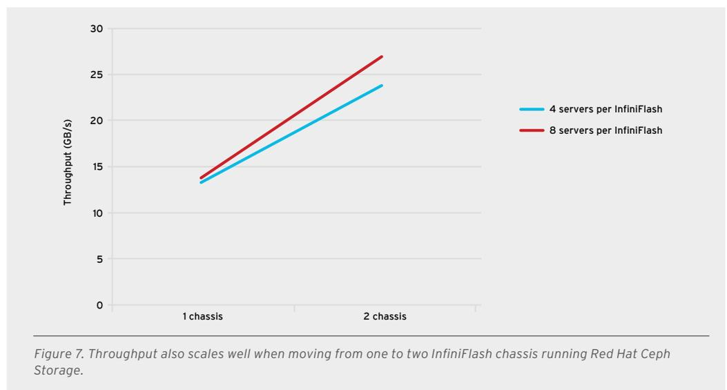
These two graphs illustrate the flexibility of InfiniFlash to vary the ratio between storage compute and storage capacity to fit workload needs. Figure 6 illustrates significantly higher IOPS performance by doubling the amount of storage compute per InfiniFlash chassis. On the other hand, throughput-intensive workloads do not benefit much from adding additional compute resources, as illustrated in Figure 7.
