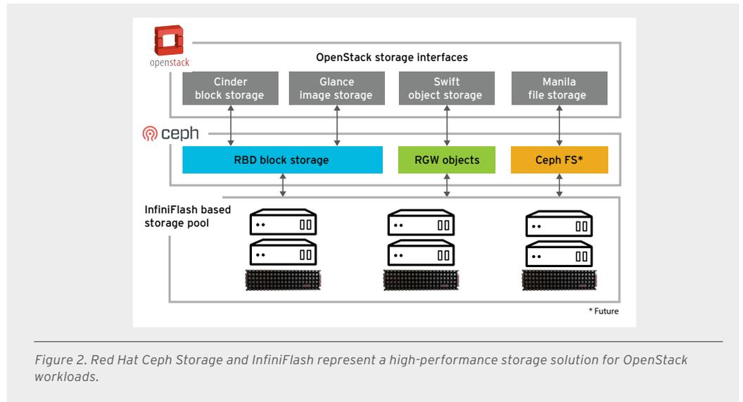
Figure 2. Red Hat Ceph Storage and InfiniFlash represent a high-performance storage solution for OpenStack workloads.
