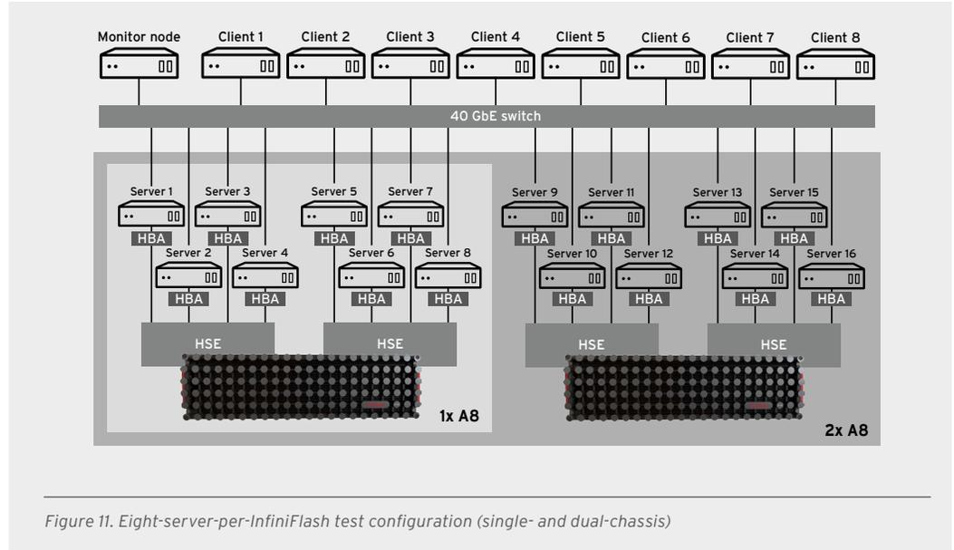
Figure 11. Eight-server-per-InfiniFlash test configuration (single- and dual-chassis)
