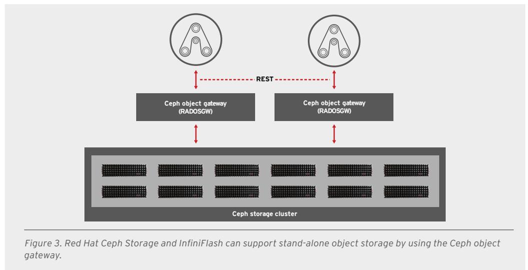
Figure 3. Red Hat Ceph Storage and InfiniFlash can support stand-alone object storage by using the Ceph object gateway.
