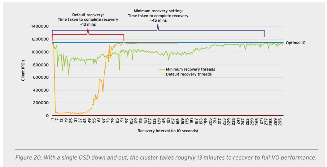
Figure 20. With a single OSD down and out, the cluster takes roughly 13 minutes to recover to full I/O performance.
